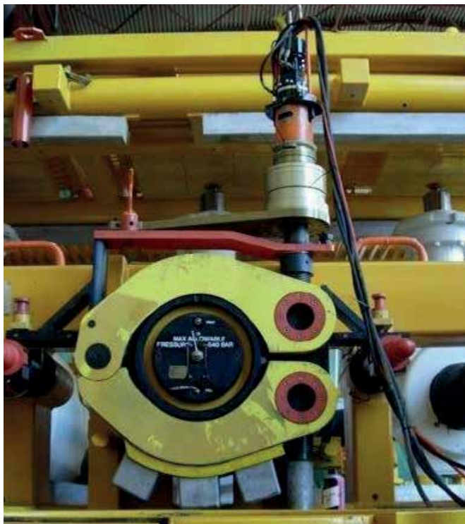
Wet Pipe Clamp Tool under test
