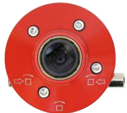
AWUR Set to clockwise operation
